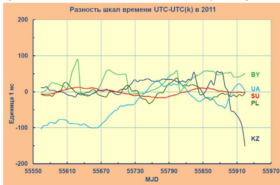
Fig. 1. An interposition of time scales of the COOMET-laboratories in 2011 with regard to the international UTC time scale obtained by GPS signal comparisons.
